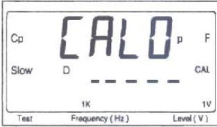
This calibration takes about 10 seconds. After it is finished, the **PeakTech**<sup>®</sup> 2150 will beep to show, that the calibration is done.
