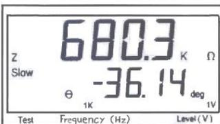
The testing level and frequency can be selected by pressing the LEVEL-key and FREQUENCY-key, respectively.
