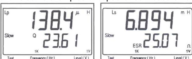
The testing level and frequency can be selected by pressing the LEVEL-key and FREQUENCY-key, respectively.
